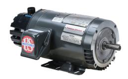
U.S. MOTORS ACCU-Torq premium efficiency AC induction motor, high-performance inverter duty, 1/4hp, 3-phase, 230/460 VAC, 1800rpm, TENV, NEMA 56C frame, rolled steel, C-face/rigid base mount. Avtron HS35A encoder included.
