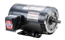
U.S. MOTORS ACCU-Torq premium efficiency AC induction motor, high-performance inverter duty, 1/2hp, 3-phase, 230/460 VAC, 1800rpm, TENV, NEMA 56C frame, rolled steel, C-face/rigid base mount.
