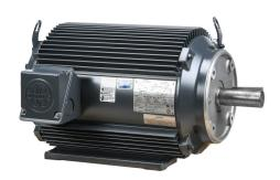
U.S. MOTORS ACCU-Torq premium efficiency AC induction motor, high-performance inverter duty, 10hp, 3-phase, 230/460 VAC, 1200rpm, TENV, NEMA 256TC frame, aluminum, C-face/rigid base mount.
