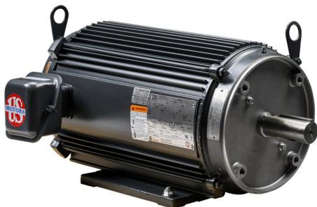
U.S. MOTORS ACCU-Torq premium efficiency AC induction motor, high-performance inverter duty, 10hp, 3-phase, 230/460 VAC, 1800rpm, TENV, NEMA 215TC frame, aluminum, C-face/rigid base mount.
