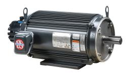
U.S. MOTORS ACCU-Torq premium efficiency AC induction motor, high-performance inverter duty, 10hp, 3-phase, 230/460 VAC, 1800rpm, TENV, NEMA 215TC frame, aluminum, C-face/rigid base mount. Avtron HS35A encoder included.
