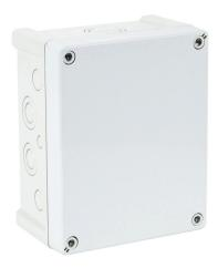
Fibox TEMPO series enclosure, NEMA 1/4/4X, 201 x 163 x 98 mm (HxWxD), polycarbonate, RAL 7035 light gray, hinged screw cover, purchase subpanel separately.
