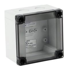
Fibox MNX series enclosure, NEMA 1/4/4X/6,  $100 \times 100 \times 60 \text{ mm}$  (HxWxD), polycarbonate, RAL 7035 light gray, smoke screw cover, purchase subpanel separately.
