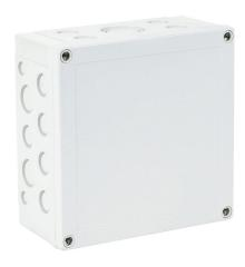
Fibox MNX series enclosure, NEMA 1/4/4X/6, 180 x 180 x 85 mm (HxWxD), polycarbonate, RAL 7035 light gray, screw cover, purchase subpanel separately.
