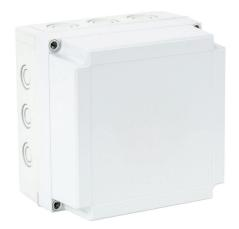
Fibox MNX series enclosure, NEMA 1/4/4X/6, 180 x 180 x 125 mm (HxWxD), polycarbonate, RAL 7035 light gray, screw cover, purchase subpanel separately.
