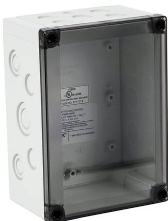
Fibox MNX series enclosure, NEMA 1/4/4X/6, 180 x 130 x 85 mm (HxWxD), polycarbonate, RAL 7035 light gray, smoke screw cover, purchase subpanel separately.
