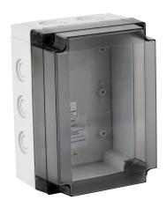
Fibox MNX series enclosure, NEMA 1/4/4X/6,  $180 \times 130 \times 100$  mm (HxWxD), polycarbonate, RAL 7035 light gray, smoke screw cover, purchase subpanel separately.
