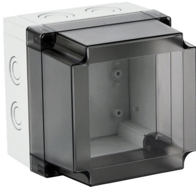
Fibox MNX series enclosure, NEMA 1/4/4X/6, 130 x 130 x 125 mm (HxWxD), polycarbonate, RAL 7035 light gray, smoke screw cover, purchase subpanel separately.
