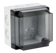
Fibox MNX series enclosure, NEMA 1/4/4X/6, 130 x 130 x 100 mm (HxWxD), polycarbonate, RAL 7035 light gray, smoke screw cover, purchase subpanel separately.
