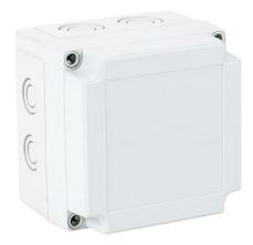
Fibox MNX series enclosure, NEMA 1/4/4X/6,  $130 \times 130 \times 100$  mm (HxWxD), polycarbonate, RAL 7035 light gray, screw cover, purchase subpanel separately.
