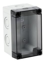
Fibox MNX series enclosure, NEMA 1/4/4X/6, 130 x 80 x 75 mm (HxWxD), polycarbonate, RAL 7035 light gray, smoke screw cover, purchase subpanel separately.
