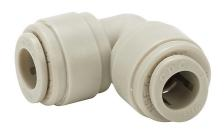
HydroMode potable water push-to-connect fitting, union elbow, acetal body, (2) 5/16in tube connection(s), NSF/ANSI 61. Package of 5.
