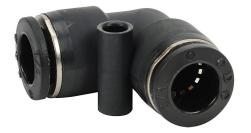
NITRA pneumatic push-to-connect fitting, union elbow, thermoplastic (PBT) body, (2) 3/8in tube connection(s). Package of 5.
