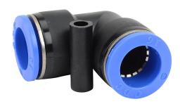
NITRA pneumatic push-to-connect fitting, union elbow, thermoplastic (PBT) body, (1) 16mm push-to-connect to (1) 16mm push-to-connect. Package of 5.
