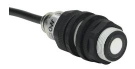
Micro Detectors ultrasonic proximity sensor, tubular, 18mm diameter x 54.9mm body, polybutylene terephthalate housing, PNP, N.O./N.C. selectable output, 60-800mm sensing distance, 6 Hz switching frequency, IP67, pigtail.
