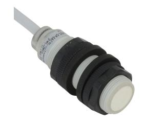
Micro Detectors ultrasonic proximity sensor, tubular, 18mm diameter x 54.9mm body, polybutylene terephthalate housing, PNP, N.O./N.C. selectable output, 60-800mm sensing distance, 6 Hz switching frequency, IP67, pigtail.
