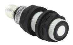
Micro Detectors ultrasonic proximity sensor, tubular, 18mm diameter x 60.4mm body, polybutylene terephthalate housing, NPN, N.O./N.C. selectable output, 60-800mm sensing distance, 6 Hz switching frequency, IP67, 4-pin M12 quick-disconnect.
