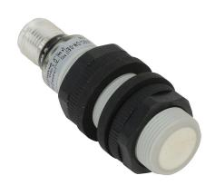
Micro Detectors ultrasonic proximity sensor, tubular, 18mm diameter x 60.4mm body, polybutylene terephthalate housing, NPN, N.O./N.C. selectable output, 60-800mm sensing distance, 6 Hz switching frequency, IP67, 4-pin M12 quick-disconnect.
