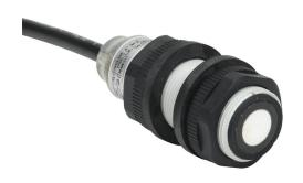
Micro Detectors ultrasonic proximity sensor, tubular, 18mm diameter x 54.9mm body, polybutylene terephthalate housing, NPN, N.O./N.C. selectable output, 60-800mm sensing distance, 6 Hz switching frequency, IP67, pigtail.
