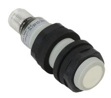
Micro Detectors ultrasonic proximity sensor, tubular, 18mm diameter x 60.4mm body, polybutylene terephthalate housing, 4-20 mA analog output, 60-800mm sensing distance, 6 Hz switching frequency, IP67, 4-pin M12 quick-disconnect.
