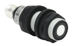
Micro Detectors ultrasonic proximity sensor, tubular, 18mm diameter x 60.4mm body, polybutylene terephthalate housing, 4-20 mA analog output, 60-800mm sensing distance, 6 Hz switching frequency, IP67, 4-pin M12 quick-disconnect.
