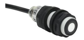
Micro Detectors ultrasonic proximity sensor, tubular, 18mm diameter x 54.9mm body, polybutylene terephthalate housing, 4-20 mA analog output, 60-800mm sensing distance, 6 Hz switching frequency, IP67, pigtail.
