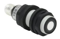
Micro Detectors ultrasonic proximity sensor, tubular, 18mm diameter x 60.4mm body, polybutylene terephthalate housing, 0-10 VDC analog output, 60-800mm sensing distance, 6 Hz switching frequency, IP67, 4-pin M12 quick-disconnect.
