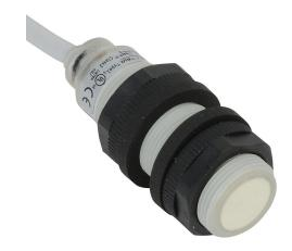
Micro Detectors ultrasonic proximity sensor, tubular, 18mm diameter x 54.9mm body, polybutylene terephthalate housing, 0-10 VDC analog output, 60-800mm sensing distance, 6 Hz switching frequency, IP67, pigtail.
