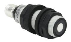
Micro Detectors ultrasonic proximity sensor, tubular, 18mm diameter x 60.4mm body, polybutylene terephthalate housing, PNP, N.O./N.C. selectable output, 40-300mm sensing distance, 12 Hz switching frequency, IP67, 4-pin M12 quick-disconnect.
