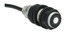
Micro Detectors ultrasonic proximity sensor, tubular, 18mm diameter x 54.9mm body, polybutylene terephthalate housing, PNP, N.O./N.C. selectable output, 40-300mm sensing distance, 12 Hz switching frequency, IP67, pigtail.
