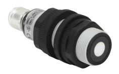
Micro Detectors ultrasonic proximity sensor, tubular, 18mm diameter x 60.4mm body, polybutylene terephthalate housing, NPN, N.O./N.C. selectable output, 40-300mm sensing distance, 12 Hz switching frequency, IP67, 4-pin M12 quick-disconnect.
