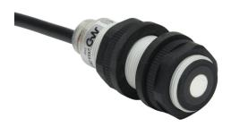
Micro Detectors ultrasonic proximity sensor, tubular, 18mm diameter x 54.9mm body, polybutylene terephthalate housing, NPN, N.O./N.C. selectable output, 40-300mm sensing distance, 12 Hz switching frequency, IP67, pigtail.
