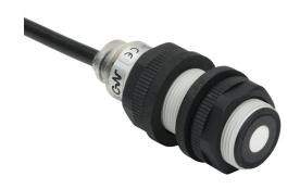
Micro Detectors ultrasonic proximity sensor, tubular, 18mm diameter x 54.9mm body, polybutylene terephthalate housing, 4-20 mA analog output, 40-300mm sensing distance, 12 Hz switching frequency, IP67, pigtail.
