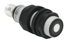
Micro Detectors ultrasonic proximity sensor, tubular, 18mm diameter x 60.4mm body, polybutylene terephthalate housing, 0-10 VDC analog output, 40-300mm sensing distance, 12 Hz switching frequency, IP67, 4-pin M12 quick-disconnect.
