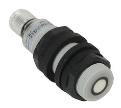
Micro Detectors ultrasonic proximity sensor, tubular, 18mm diameter x 60.4mm body, polybutylene terephthalate housing, 0-10 VDC analog output, 40-300mm sensing distance, 12 Hz switching frequency, IP67, 4-pin M12 quick-disconnect.
