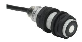
Micro Detectors ultrasonic proximity sensor, tubular, 18mm diameter x 54.9mm body, polybutylene terephthalate housing, 0-10 VDC analog output, 40-300mm sensing distance, 12 Hz switching frequency, IP67, pigtail.
