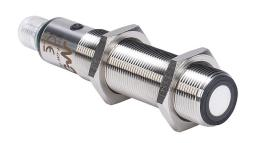
Micro Detectors ultrasonic proximity sensor, tubular, 18mm diameter x 91.6mm body, 316L stainless steel housing, PNP, (2) N.O./N.C. selectable outputs, 200-2200mm sensing distance, 2 Hz switching frequency, IP67, 5-pin M12 quick-disconnect.
