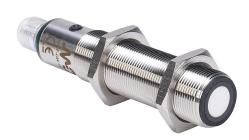
Micro Detectors ultrasonic proximity sensor, tubular, 18mm diameter x 91.6mm body, 316L stainless steel housing, PNP, (2) N.O./N.C. selectable outputs, 200-2200mm sensing distance, 2 Hz switching frequency, IP67, 5-pin M12 quick-disconnect.
