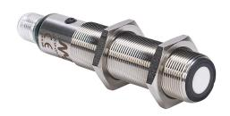
Micro Detectors ultrasonic proximity sensor, tubular, 18mm diameter x 91.6mm body, 316L stainless steel housing, PNP, N.O./ N.C. selectable output, 200-2200mm sensing distance, 2 Hz switching frequency, IP67, 4-pin M12 quick-disconnect.
