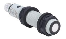
Micro Detectors ultrasonic proximity sensor, tubular, 18mm diameter x 91.6mm body, polybutylene terephthalate housing, PNP, N.O./N.C. selectable output, 200-2200mm sensing distance, 2 Hz switching frequency, IP67, 4-pin M12 quick-disconnect.
