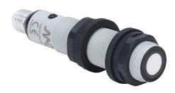
Micro Detectors ultrasonic proximity sensor, tubular, 18mm diameter x 91.6mm body, polybutylene terephthalate housing, NPN, N.O./N.C. selectable output, 200-2200mm sensing distance, 2 Hz switching frequency, IP67, 4-pin M12 quick-disconnect.
