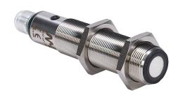
Micro Detectors ultrasonic proximity sensor, tubular, 18mm diameter x 91.6mm body, 316L stainless steel housing, PNP, 0-10 VDC analog output, N.O./N.C. selectable output, 200-2200mm sensing distance, 2 Hz switching frequency, IP67, 5-pin M12 quick-disconnect.
