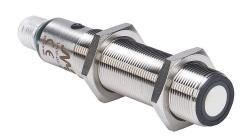
Micro Detectors ultrasonic proximity sensor, tubular, 18mm diameter x 91.6mm body, 316L stainless steel housing, 4-20 mA analog output, 200-2200mm sensing distance, 1 Hz switching frequency, IP67, 4-pin M12 quick-disconnect.
