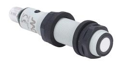
Micro Detectors ultrasonic proximity sensor, tubular, 18mm diameter x 91.6mm body, polybutylene terephthalate housing, 4-20 mA analog output, 200-2200mm sensing distance, 1 Hz switching frequency, IP67, 4-pin M12 quick-disconnect.
