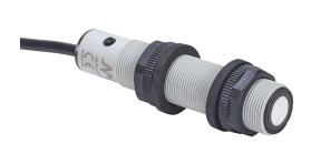
Micro Detectors ultrasonic proximity sensor, tubular, 18mm diameter x 83.6mm body, polybutylene terephthalate housing, 4-20 mA analog output, 200-2200mm sensing distance, 1 Hz switching frequency, IP67, pigtail.
