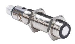
Micro Detectors ultrasonic proximity sensor, tubular, 18mm diameter x 91.6mm body, 316L stainless steel housing, 0-10 VDC analog output, 200-2200mm sensing distance, 1 Hz switching frequency, IP67, 4-pin M12 quick-disconnect.
