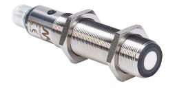
Micro Detectors ultrasonic proximity sensor, tubular, 18mm diameter x 91.6mm body, 316L stainless steel housing, PNP, (2) N.O./N.C. selectable outputs, 150-1600mm sensing distance, 3 Hz switching frequency, IP67, 5-pin M12 quick-disconnect.
