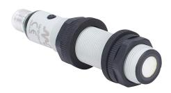
Micro Detectors ultrasonic proximity sensor, tubular, 18mm diameter x 91.6mm body, polybutylene terephthalate housing, PNP, (2) N.O./N.C. selectable outputs, 150-1600mm sensing distance, 3 Hz switching frequency, IP67, 5-pin M12 quick-disconnect.
