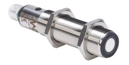
Micro Detectors ultrasonic proximity sensor, tubular, 18mm diameter x 91.6mm body, 316L stainless steel housing, PNP, N.O./ N.C. selectable output, 150-1600mm sensing distance, 3 Hz switching frequency, IP67, 4-pin M12 quick-disconnect.
