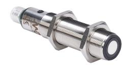
Micro Detectors ultrasonic proximity sensor, tubular, 18mm diameter x 91.6mm body, 316L stainless steel housing, PNP, N.O./ N.C. selectable output, 150-1600mm sensing distance, 3 Hz switching frequency, IP67, 4-pin M12 quick-disconnect.
