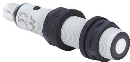
Micro Detectors ultrasonic proximity sensor, tubular, 18mm diameter x 91.6mm body, polybutylene terephthalate housing, PNP, N.O./N.C. selectable output, 150-1600mm sensing distance, 3 Hz switching frequency, IP67, 4-pin M12 quick-disconnect.
