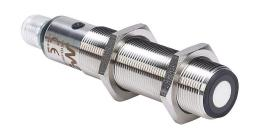
Micro Detectors ultrasonic proximity sensor, tubular, 18mm diameter x 91.6mm body, 316L stainless steel housing, NPN, N.O./ N.C. selectable output, 150-1600mm sensing distance, 3 Hz switching frequency, IP67, 4-pin M12 quick-disconnect.
