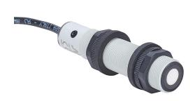
Micro Detectors ultrasonic proximity sensor, tubular, 18mm diameter x 83.6mm body, polybutylene terephthalate housing, NPN, N.O./N.C. selectable output, 150-1600mm sensing distance, 3 Hz switching frequency, IP67, pigtail.
