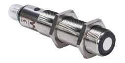
Micro Detectors ultrasonic proximity sensor, tubular, 18mm diameter x 91.6mm body, 316L stainless steel housing, PNP, 0-10 VDC analog output, N.O./N.C. selectable output, 150-1600mm sensing distance, 3 Hz switching frequency, IP67, 5-pin M12 quick-disconnect.
