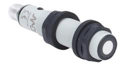
Micro Detectors ultrasonic proximity sensor, tubular, 18mm diameter x 91.6mm body, polybutylene terephthalate housing, PNP, 0-10 VDC analog output, N.O./N.C. selectable output, 150-1600mm sensing distance, 3 Hz switching frequency, IP67, 5-pin M12 quick-disconnect.
