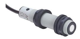
Micro Detectors ultrasonic proximity sensor, tubular, 18mm diameter x 83.6mm body, polybutylene terephthalate housing, PNP, 0-10 VDC analog output, N.O./N.C. selectable output, 150-1600mm sensing distance, 3 Hz switching frequency, IP67, pigtail.
